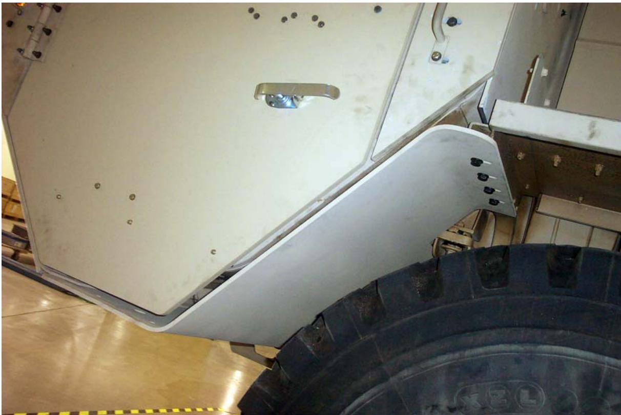
Figure 38. Install the driver's-side front blast deflector (P/N 106717-1).
