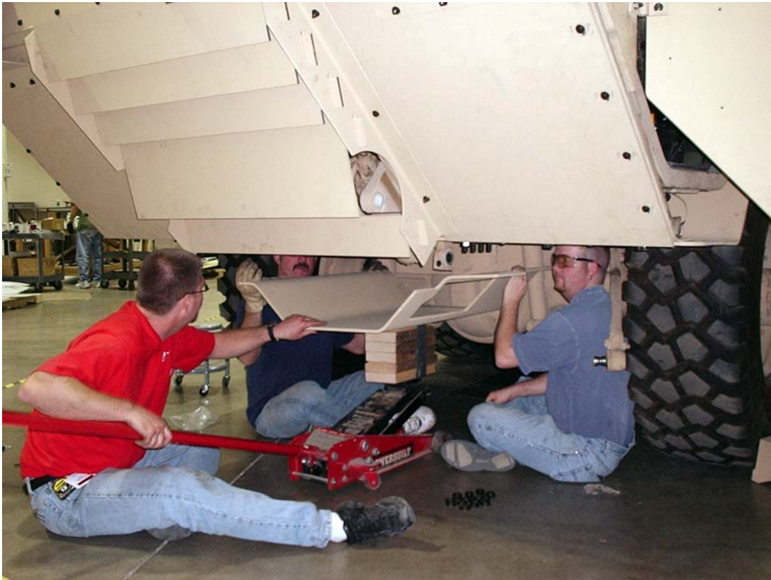
Figure 39. Position the Center Blast Deflector onto the Mounting Bracket Studs.
