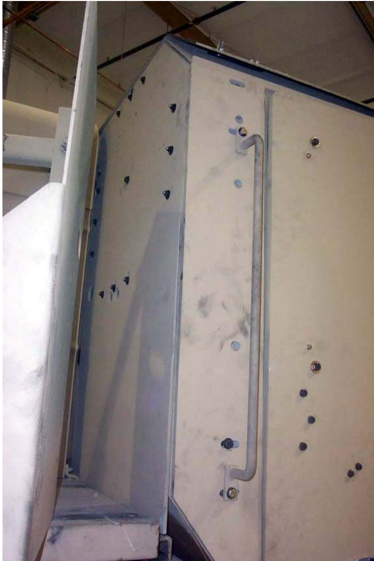
Figure 35a. The Rear Side Cab Armor Panel installed.
