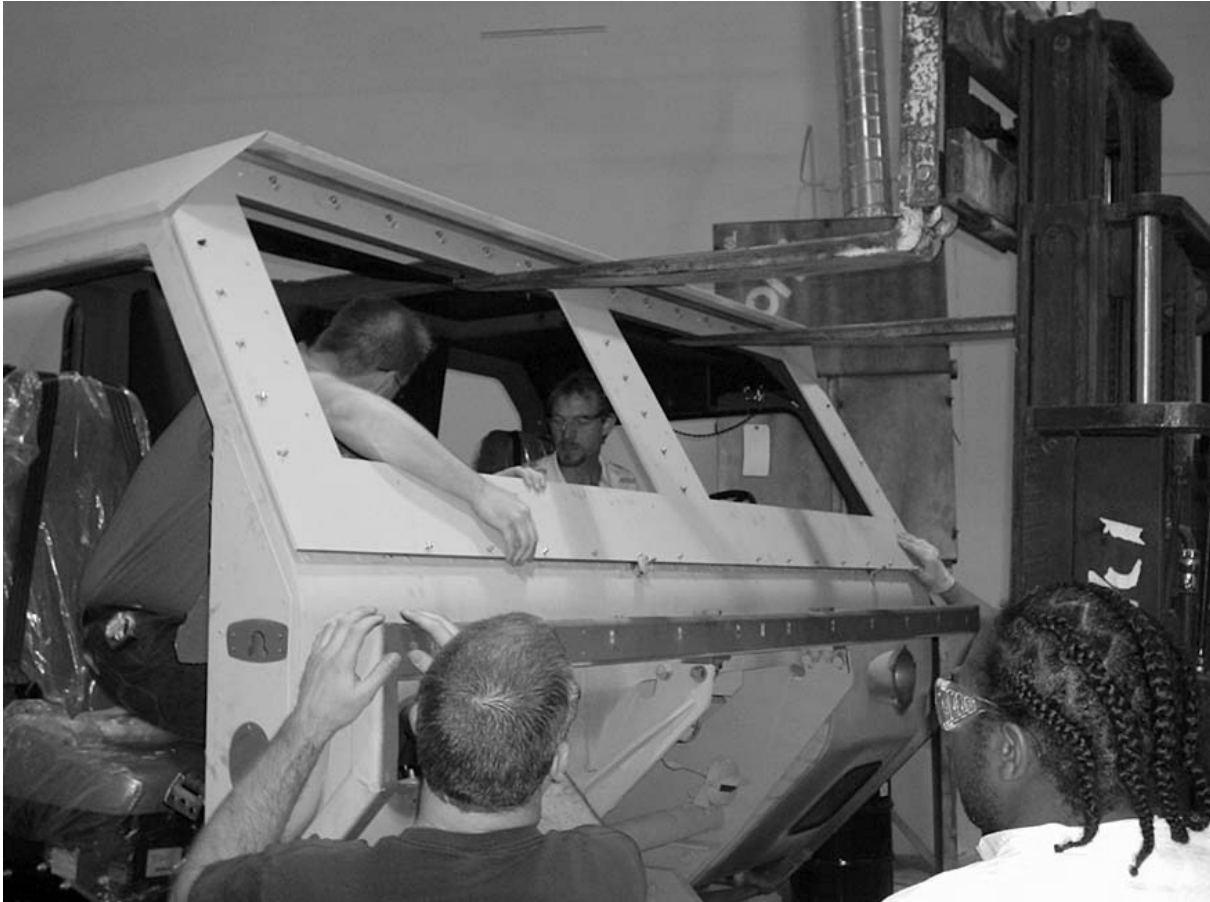
Figure 18. Position the Windshield Armor Frame into the cab windshield opening.
