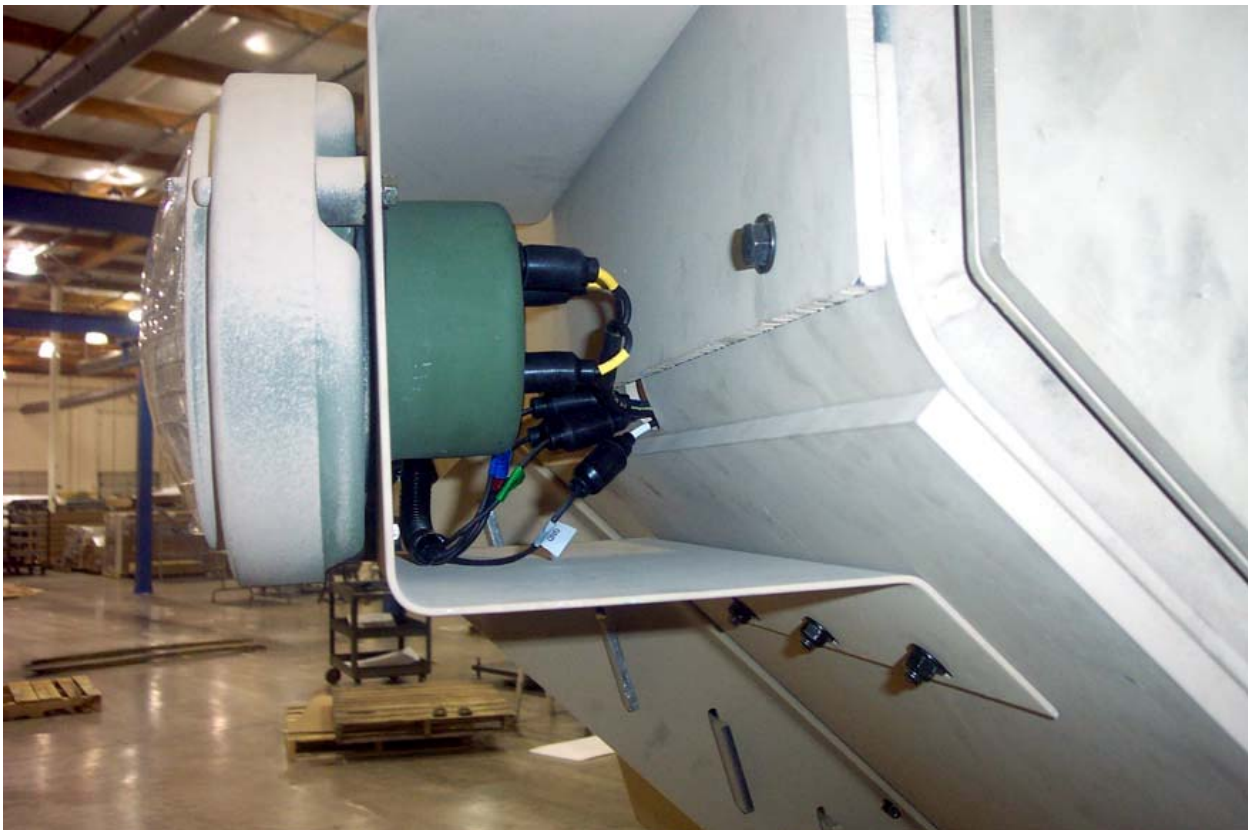
Figure 28. Left-hand Headlight Bracket Installed.
